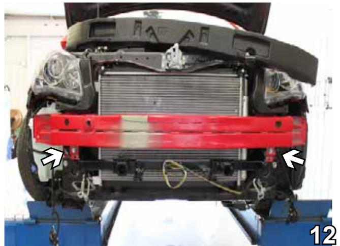
11. Again, using the baseplate as a template, drill the two side holes through the bumper on both sides using a 13/32" drill bit. Insert a 3/8-16 x 1 1/2" hex bolt with a 3/8" lock washer and a 1/4 x 1 x 1" nut plate. Tighten with Loctite Red. Do this on both sides of the vehicle.
