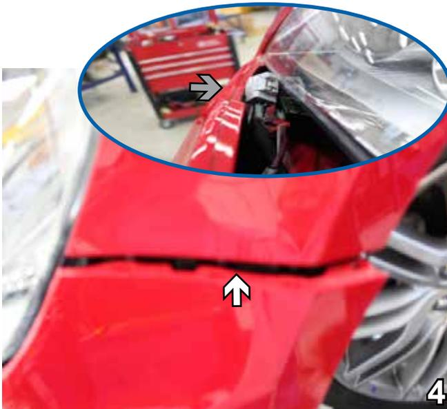
4. To remove the fascia, lift up and out on the fascia near each front tire (white arrow). To disconnect the fascia, unplug the white electrical connection located below each headlight (gray arrow). Set fascia aside to be reinstalled later.
