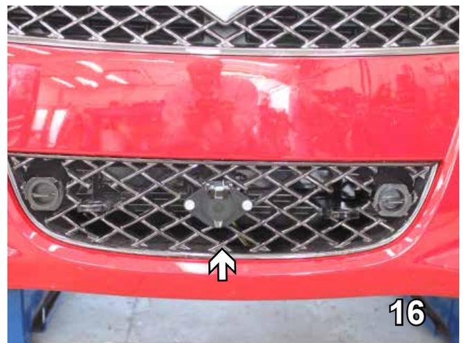
16. Reinstall the fascia, belly pan and all electrical connections using the existing bolts and push pins. Optional: Attach the electrical bracket to the center of the fascia (white arrow).
