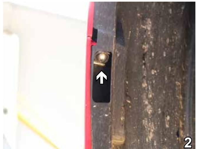
2. Use a Phillips screw driver and remove the screw concealed in the front of the wheel well. Do this on both sides of the vehicle. Set aside screws to be reinstalled later.
