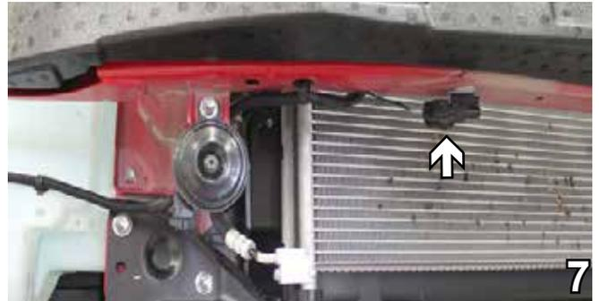
7. On the passenger's side only, disconnect the temperature sensor.
