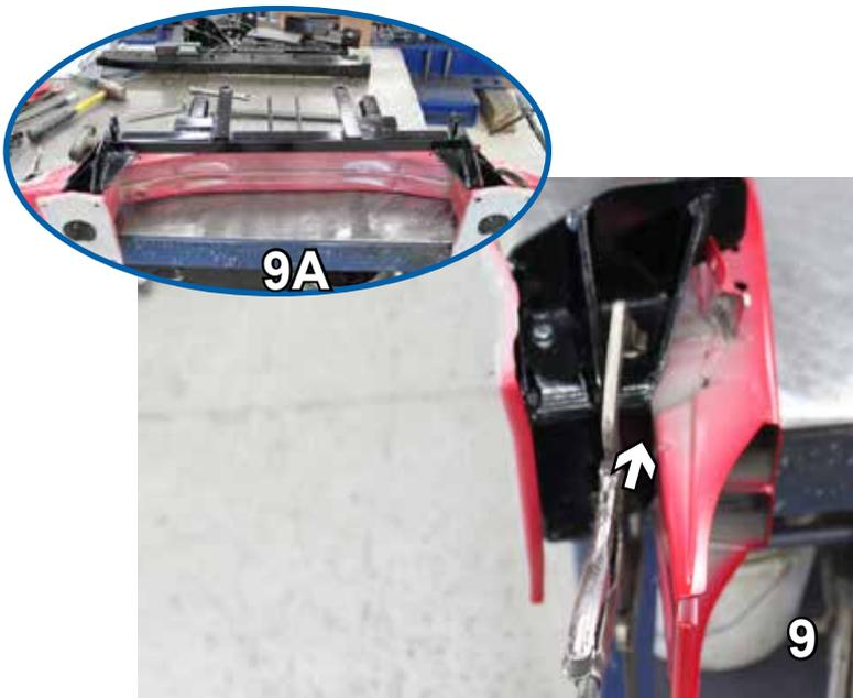
9. Placing the baseplate onto the bottom of the bumper and flush against its crossbar (9A), use a clamp to secure each side of the baseplate to the bumper's legs.
